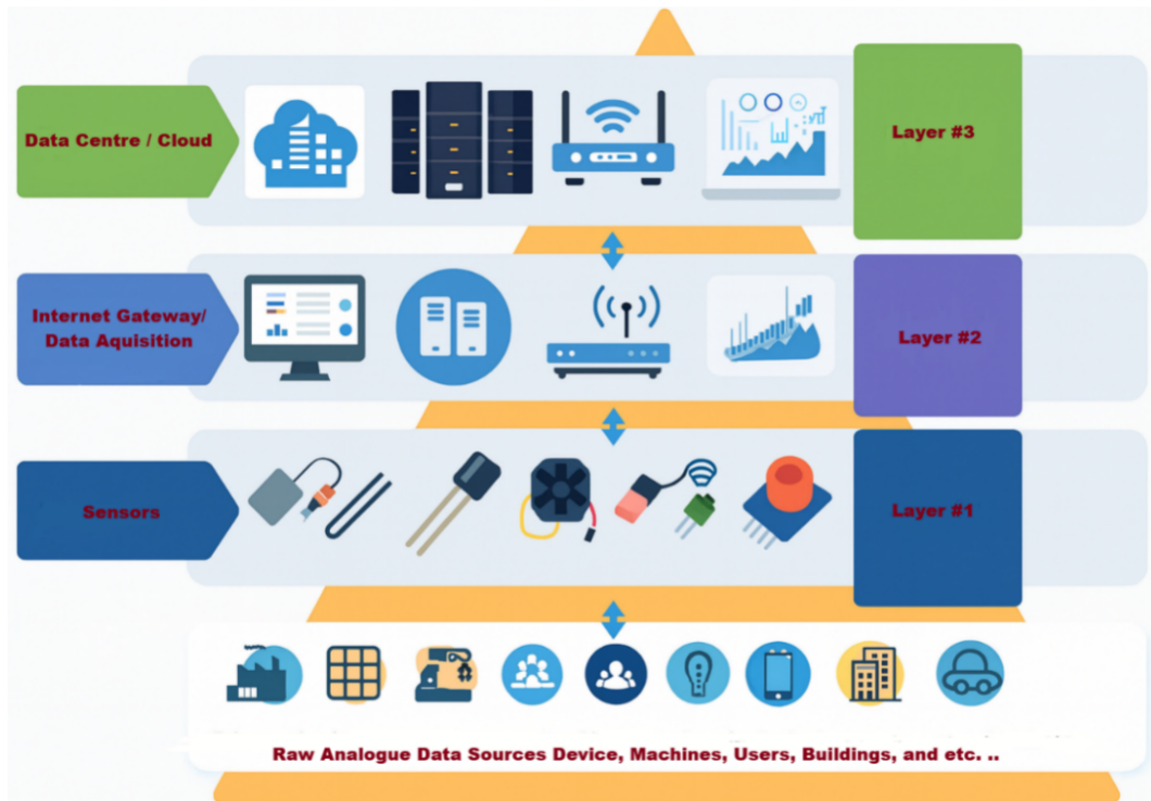
Figure 4: Layered IoT architecture for smart data acquisition and cloud integration (redrawn and adapted from [46]).
